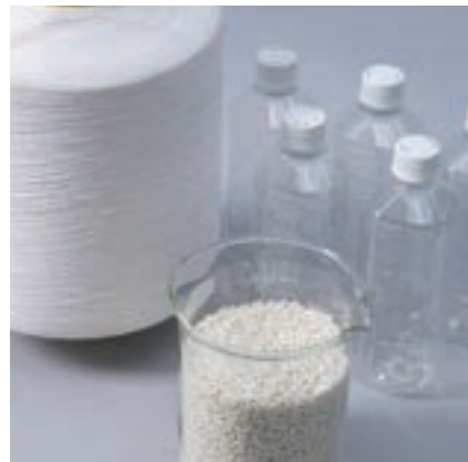
Chips made from plastic bottles become yarn
