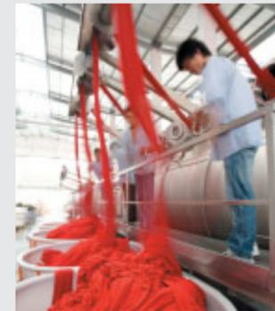
Strips of cloth joined together are dyed as they pass through the liquid flow dyeing machine.
