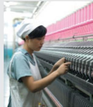
More than 10,000 cones for winding yarn must have the same degree of tension to ensure that yarn production is uniform.
