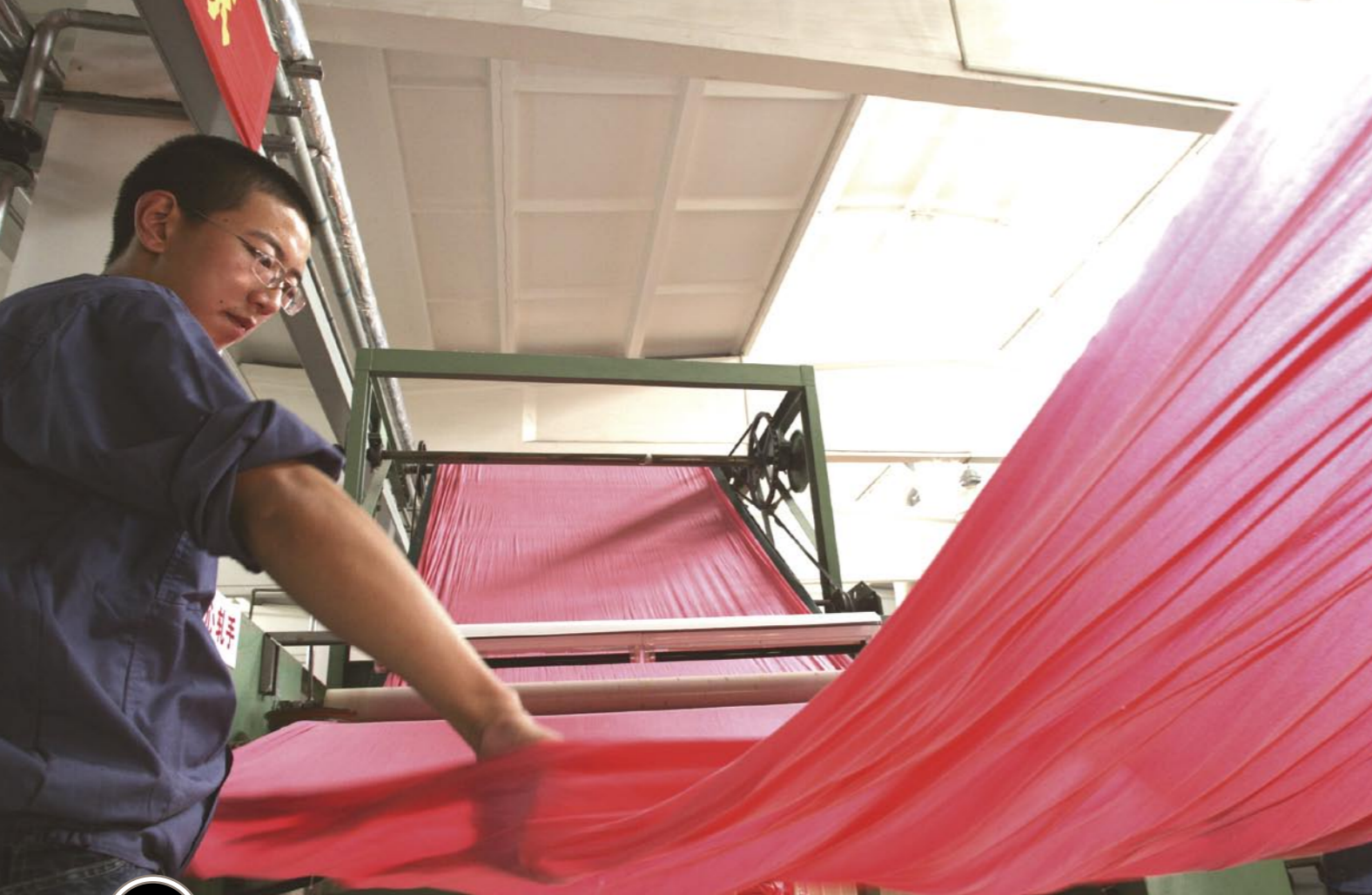
All woven clothes are inspected on a translucent light board to reveal flaws and holes before and after dyeing and before cutting
