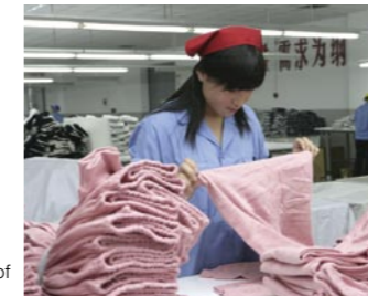
Products are stretched in sampling inspections in response to customer reports of shrinkage
