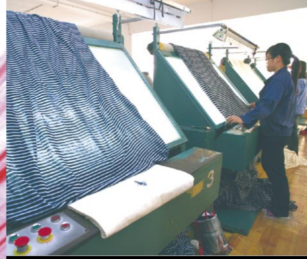
All woven clothes are inspected on a translucent light board to reveal flaws and holes before and after dyeing and before cutting
