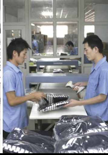
Cross-directional (vertical and horizontal) needle detection is performed
