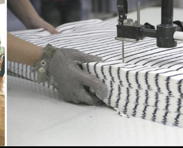
Metal gloves are required to protect workers during the cutting process
