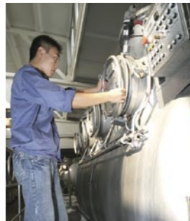
Checking dyeing conditions inside a dyeing machine
