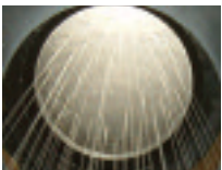
“LOC II CEO® α” filaments are extruded from a star-shaped opening, and 48 are bundled to make one HEATTECH thread.
