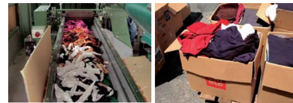
Sliced fleeces for thermal recycling
